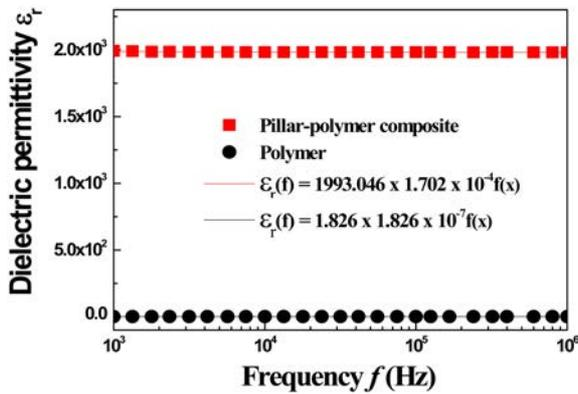
Fig. 3. Frequency-dependent relative dielectric permittivity of the PSZT ceramic pillar polymer composite and PDMS polymer.
