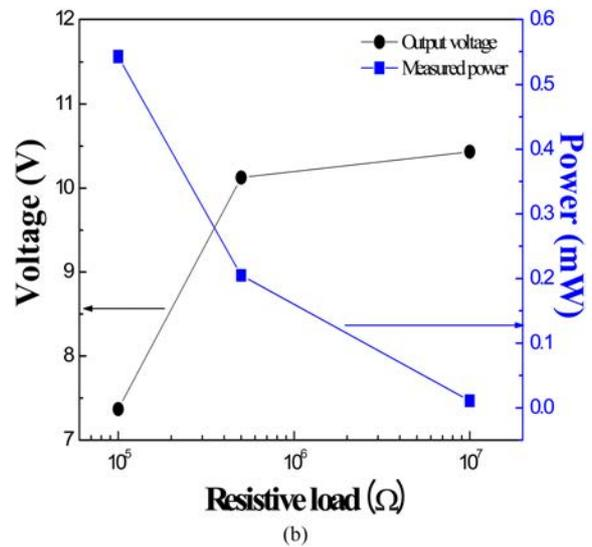
Fig. 5. Generated output voltage (a) and generated output power (b) according to the resistive load in the PSZT ceramic pillar polymer composite energy harvester.
