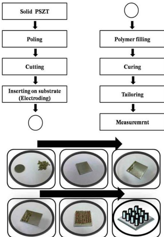
**Fig. 1.** The fabrication process for the PSZT ceramic pillar composite and its photographs.
