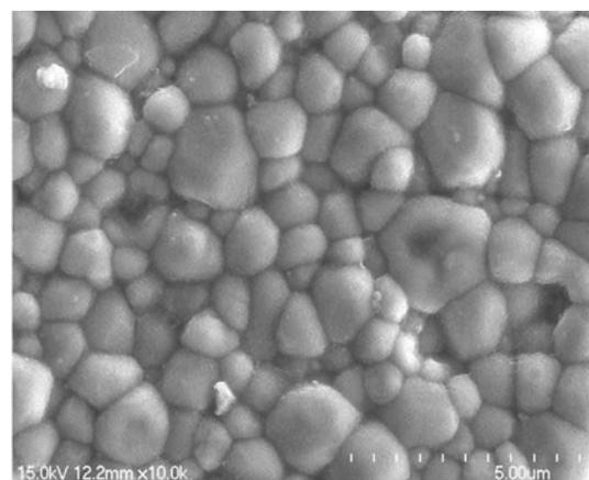
**Fig. 2.** SEM image of PSZT ceramics for the pillar structure.
