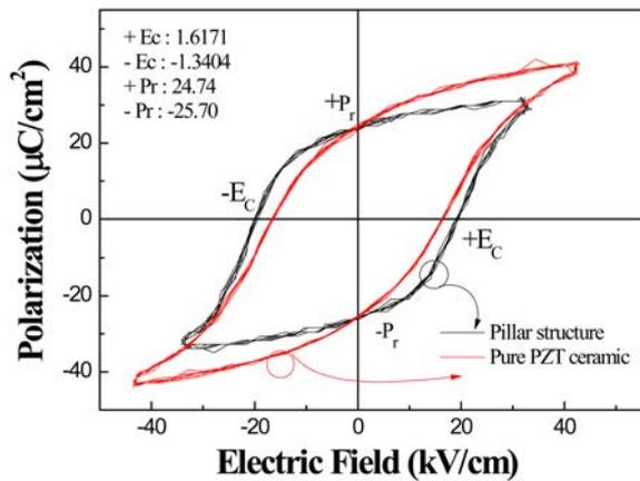
Fig. 4. The P-E hysteresis loops of the PSZT ceramic pillar polymer composite and pure PSZT ceramic bulk.
