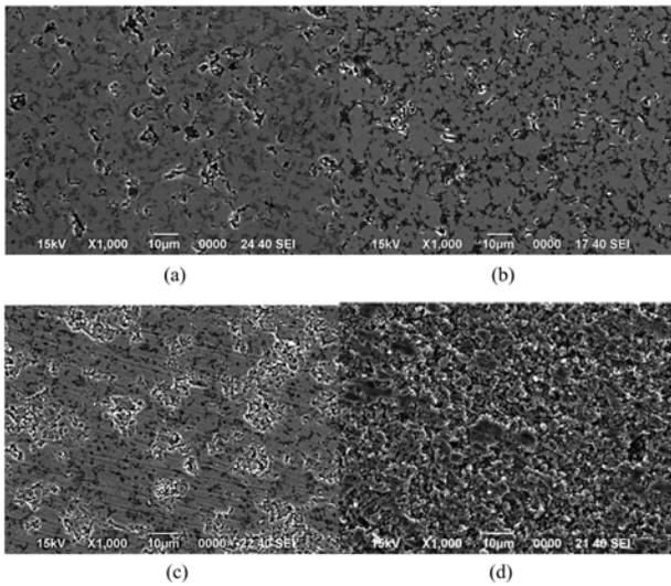
Fig. 3. The microstructures of cross sections of ribs with different porosity, (a) 0.52%, (b) 7.17%, (c) 12.10%, (d) 26.48%.
