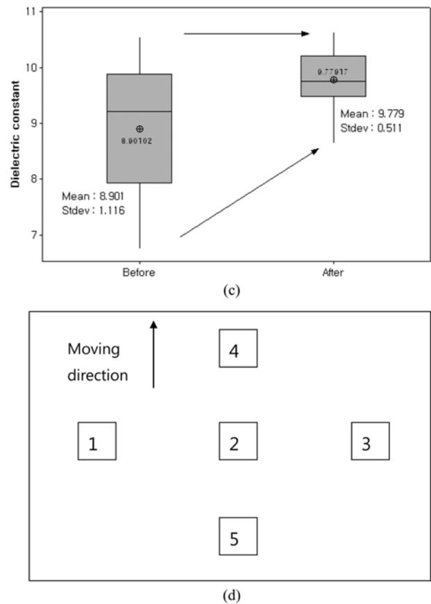
Fig. 7. The change of hardness and dielectric constant of real panels before and after improving different temperature gradients in the sintering process: (a) hardness, (b) dielectric constant according to location, (c) deviation of dielectric constant, and (d) sampling location and moving direction of the panel.
