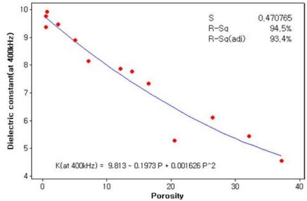
Fig. 5. The relationship between dielectric constant and porosity
