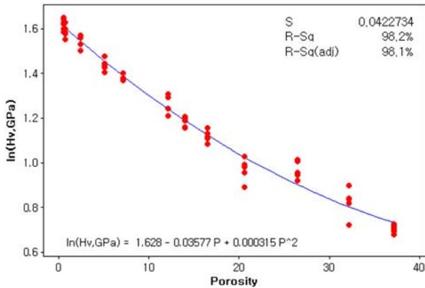
Fig. 4. The relationship between hardness and porosity.
