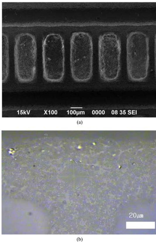
Fig. 1. The top view of barrier ribs of a 58-inch FHD TV rear panel, (a) SEM image and (b) microscope image with Vickers indentation.
