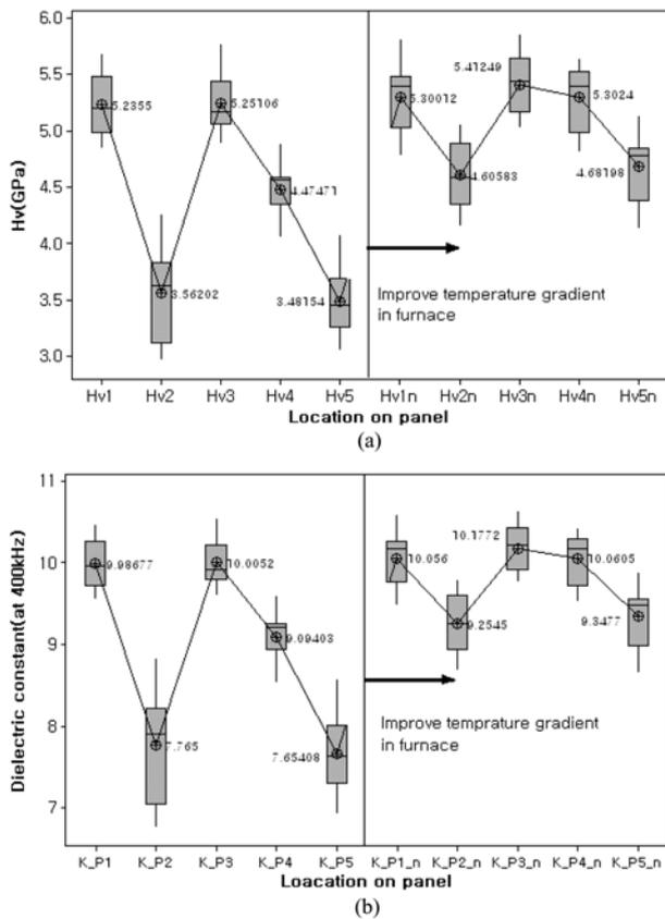
Fig. 6. The relationship between dielectric constant and hardness.
