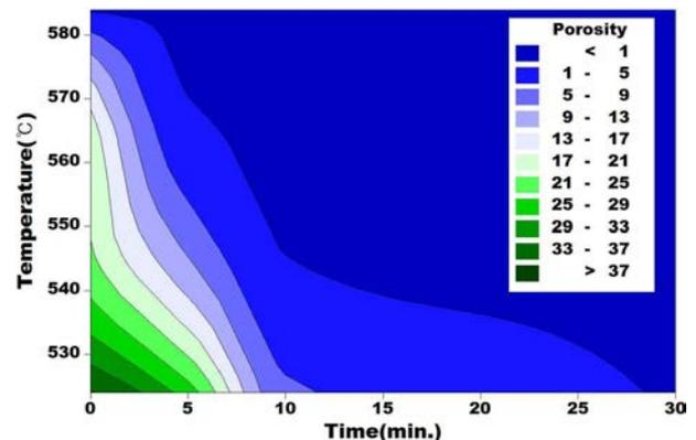
Fig. 2. The contour plot of porosity versus firing temperature and time.
