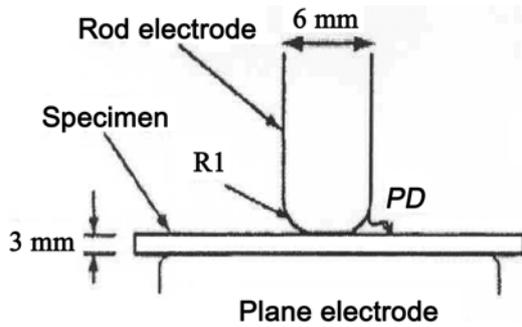
Fig. 1. IEC(b) electrode configuration for surface discharge degradation test.
