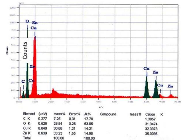
Fig. 8. Elemental composition of debris of Bakelite found at the edge of electrode.
