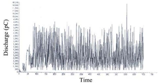
Fig. 4. Variation of PD as a function of time on the surface of PC.
