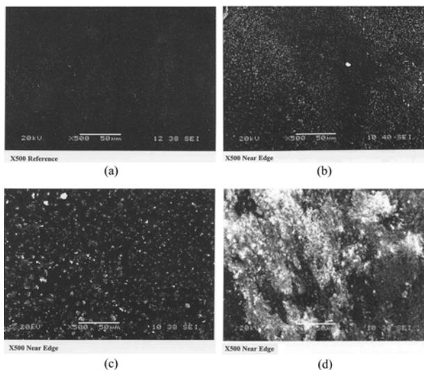
Fig. 7. Surface profile of (a) unaged sample, (b) PMMA, (c) PC, and (d) Bakelite.
