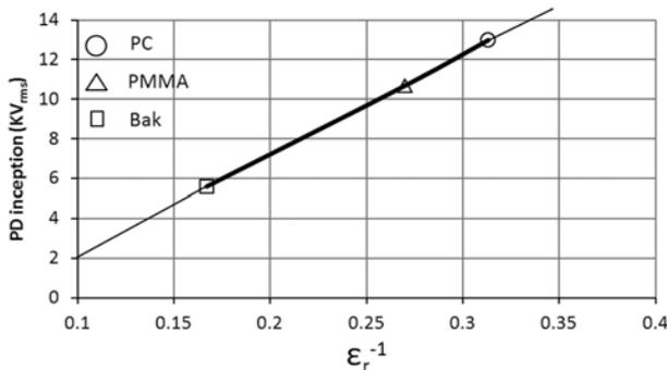
Fig. 2. PD onset voltage as a function of the reciprocal of permittivity.
