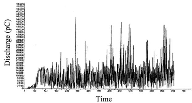
Fig. 3. Variation of PD as a function of time on the surface of Bakelite.
