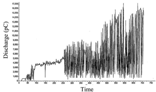
Fig. 5. Variation of PD as a function of time on the surface of PMMA.
