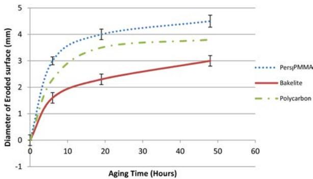
Fig. 6. Erosion diameter as a function of aging time.
