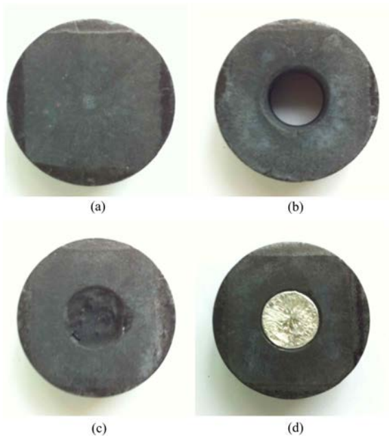
Fig. 1. The melt processed YBCO bulk; (A) without hole, (B) with hole, (C) impregnated by epoxy resin, and (d) impregnated by indium.
