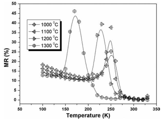
**Fig. 5.** Temperature dependence of magnetoresistance (MR%) under a magnetic field of  $H_{dc} = 1T$  for  $(La_{0.67}Ca_{0.33}MnO_3)_{0.97}/(ZnO)_{0.03}$  composites sintered at different temperature.
