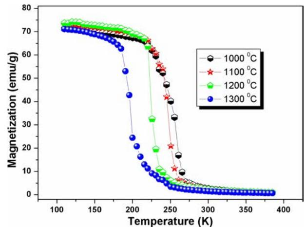
Fig. 3. Temperature dependence of magnetization of  $(\text{La}_{0.67}\text{Ca}_{0.33}\text{MnO}_3)_{0.97}/(\text{ZnO})_{0.03}$  composites sintered at different temperature.
