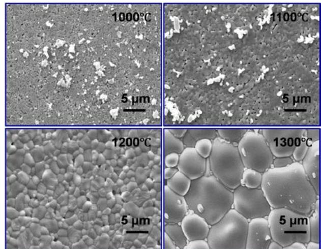
Fig. 2. SEM micrographs of  $(\text{La}_{0.67}\text{Ca}_{0.33}\text{MnO}_3)_{0.97}/(\text{ZnO})_{0.03}$  composites sintered at different temperature.
