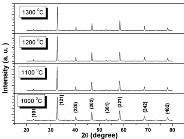
Fig. 1. X-ray diffraction patterns of  $(\text{La}_{0.67}\text{Ca}_{0.33}\text{MnO}_3)_{0.97}/(\text{ZnO})_{0.03}$  composites sintered at different temperature.
