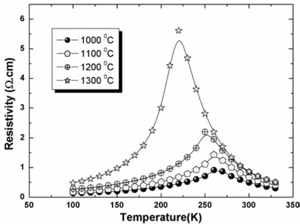
**Fig. 4.** Temperature dependence of resistivity in zero field of  $(La_{0.67}Ca_{0.33}MnO_3)_{0.97}/(ZnO)_{0.03}$  composites sintered at different temperature.
