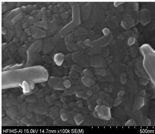
Fig. 9. FE-SEM image of sintered  $\text{Al}_2\text{TiO}_5$ .
