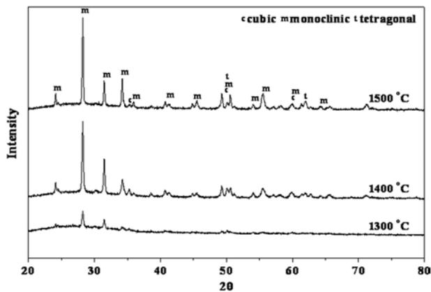
Fig. 7. XRD patterns of the sintered pellets formed from the 3YSZ powder post-treated at 900 °C.
