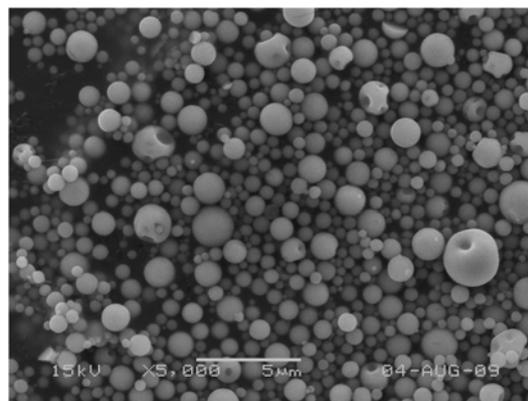
**Fig. 1.** SEM image of the precursor powders prepared from the spray solution without organic additives.
