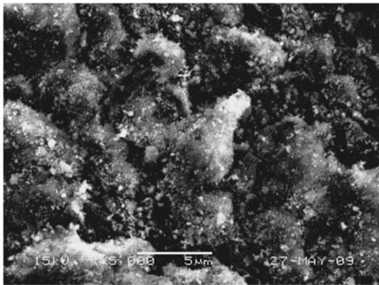
**Fig. 4.** SEM image of the post-treated 3YSZ powder obtained from the spray solution with CA and EDTA after milling.
