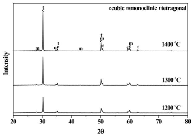
Fig. 8. XRD patterns of the sintered pellets formed from the 8YSZ powder post-treated at 900 °C.
