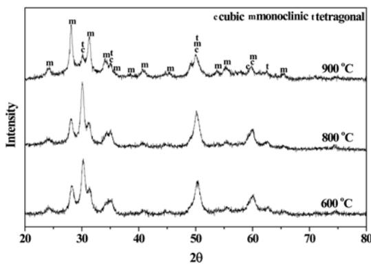
**Fig. 5.** XRD patterns of the 3YSZ powders post-treated at various temperatures.
