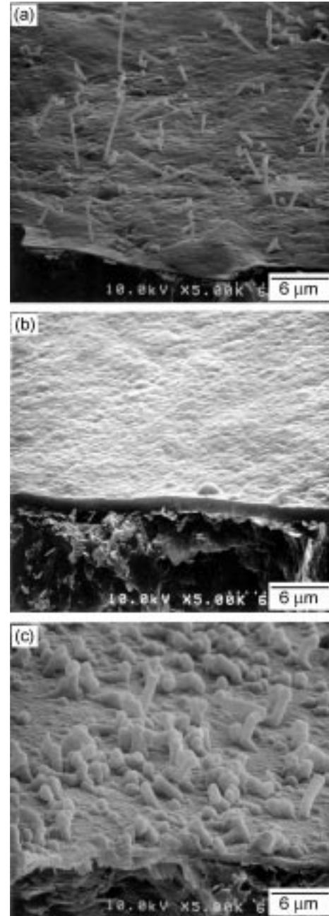
**Fig. 3.** SEM images of the deposits which were produced on graphite substrate at different deposition temperature. (a) 1000°C, (b) 1050°C, (c) 1100°C ( $\alpha=50$ ).
