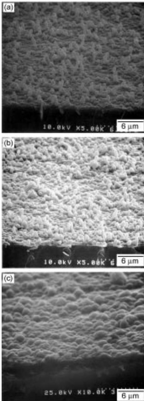
**Fig. 6.** SEM images of the deposits which were produced on Si substrates polished with #2000 SiC abrasive paper at different deposition temperatures. (a) 1000°C, (b) 1050°C, (c) 1100°C ( $\alpha=50$ ).
