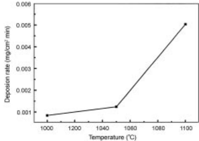
**Fig. 5.** The variation of the deposition rate as a function of deposition temperature. ( $\alpha=50$ , deposition time=2h), un-abraded and carbon coated Si substrates.
