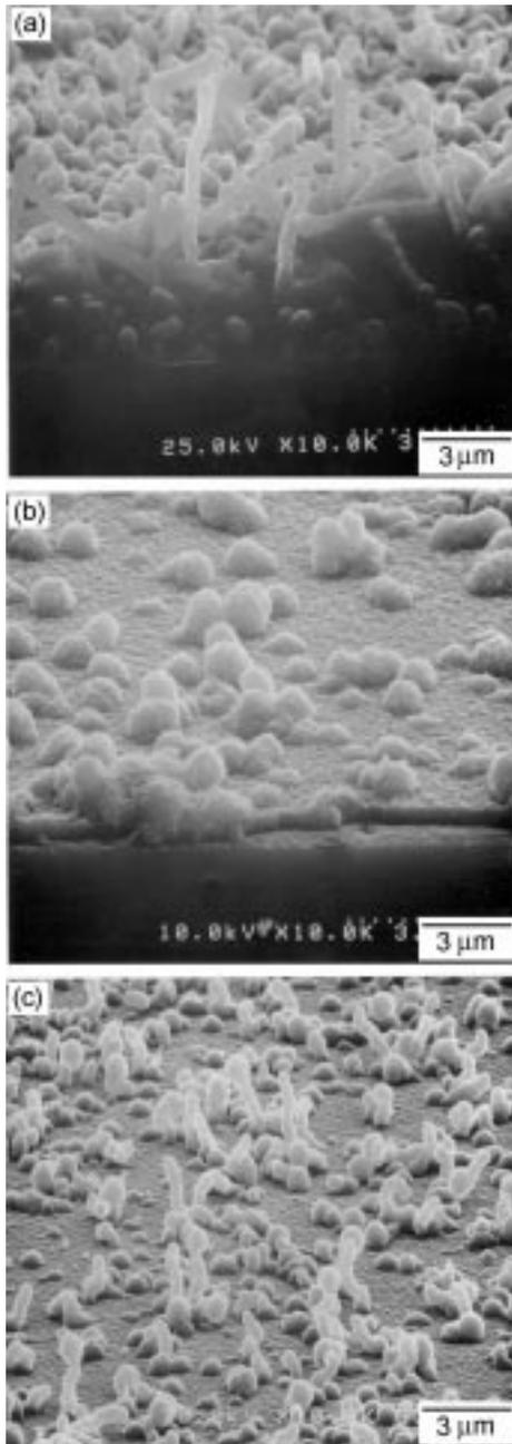
**Fig. 4.** SEM images of the deposits which were produced on un-abraded and carbon coated Si substrates at different deposition temperatures. (a) 1000°C, (b) 1050°C, (c) 1100°C ( $\alpha=50$ ).
