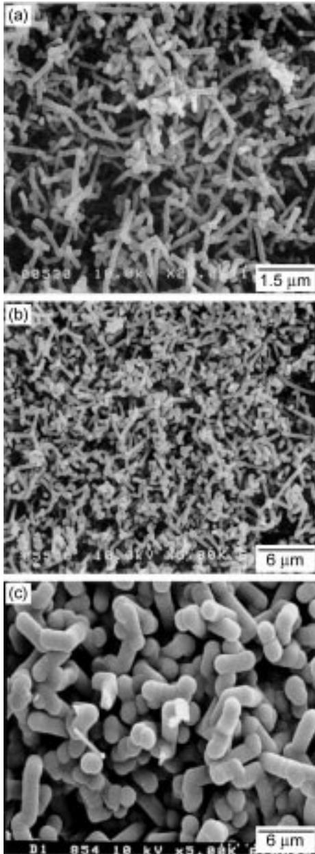
**Fig. 2.** SEM images of the deposits which were produced on graphite substrate at different deposition temperature. (a) 1000°C, (b) 1050°C, (c) 1100°C ( $\alpha=30$ ).
