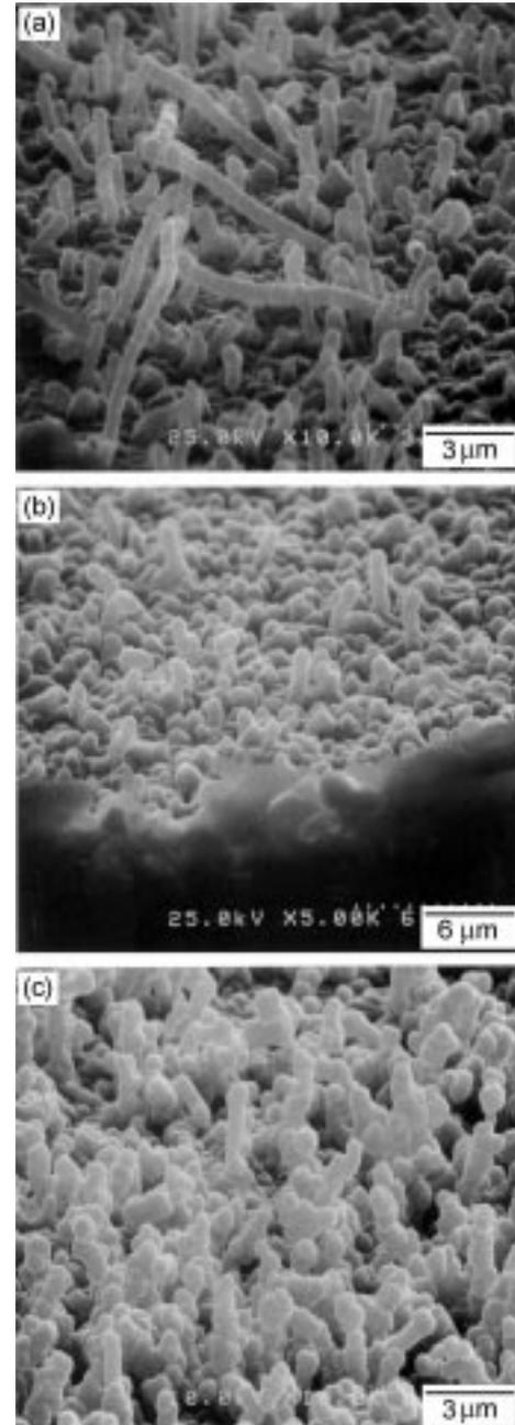
**Fig. 7.** SEM images of the deposits which were produced on Si substrates polished with #1000 SiC abrasive paper at different deposition temperatures. (a) 1000°C, (b) 1050°C, (c) 1100°C ( $\alpha=50$ ).
