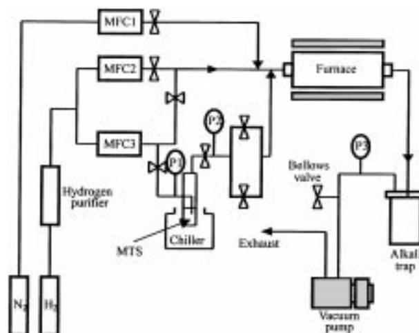
Fig. 1. The schematic diagram of a LPCVD system.
