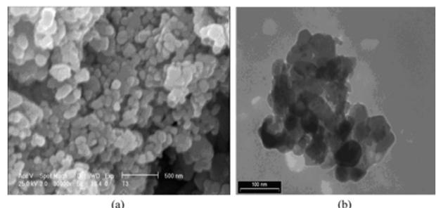
**Fig. 2.** Morphology of ZnO nano powders synthesized by a sol-gel method (a) SEM image (b) TEM image.
