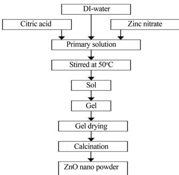
**Fig. 1.** Flow chart for synthesis of ZnO nano powder by a sol-gel method.
