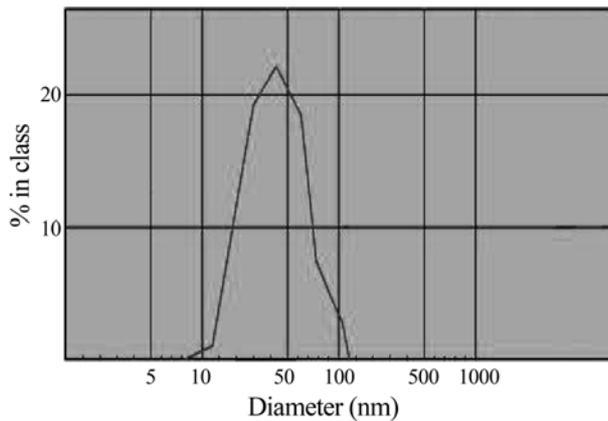
**Fig. 3.** Particle size distribution of ZnO nano powder synthesized by a sol-gel method.
