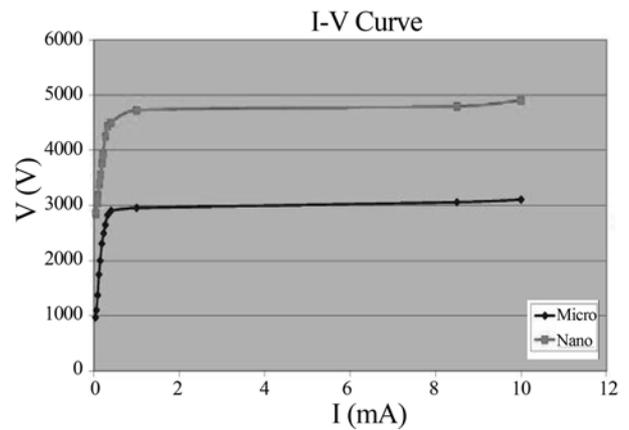
**Fig. 4.** I-V curve of varistors samples fabricated from nano and micro sized zinc oxide powders.
