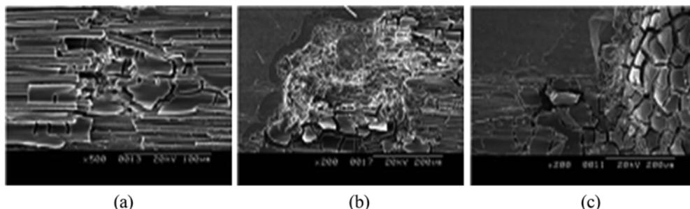
Fig. 4. The surface after crack-healing with a dip coating of SiO<sub>2</sub> nano-colloid on a cracked UCS specimen. (Crack length:(a) 215 μm, (b) 500 μm, (c) 1 mm by φ1 mm drill).
