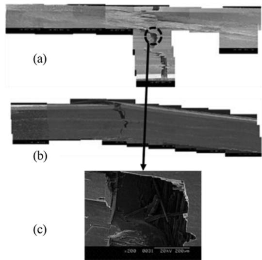
Fig. 3. SEM image of CCS after the bending test; (a) surface, (b) side, (c) enlargement of red circle (a).
