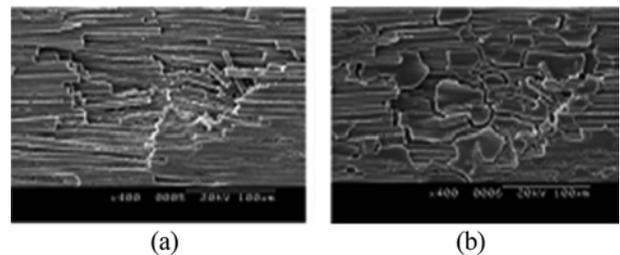
Fig. 5. The surface (a) before and (b) after crack-healing infiltrated SiO<sub>2</sub> nano-colloid with the hydrostatic pressure method on cracked UCS.
