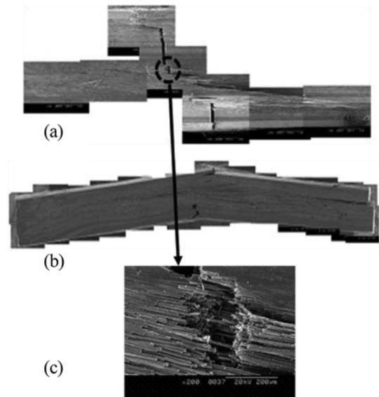
Fig. 2. SEM image of UCS after the bending test; (a) surface, (b) side, (c) enlargement of red circle (a).
