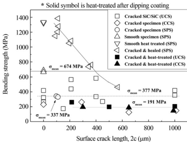
Fig. 1. Relationship between bending strength and surface crack length.
