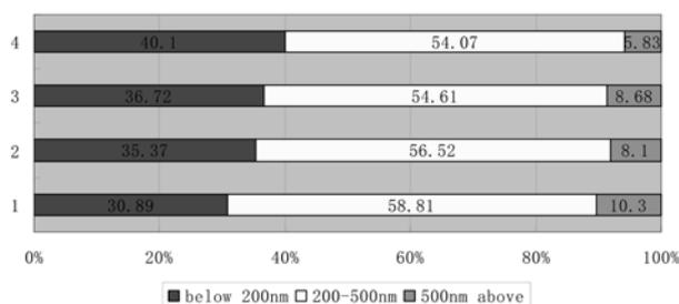
**Fig. 2.** Grain size distributions of sintered PX242A specimens with different heating rates : (1) 100°Kh<sup>-1</sup>, (2) 200°Kh<sup>-1</sup>, (3) 400°Kh<sup>-1</sup> and (4) 600°Kh<sup>-1</sup>.**Table 2.** Average and standard deviation of total transmission, transparency parameter and contrast ratio
