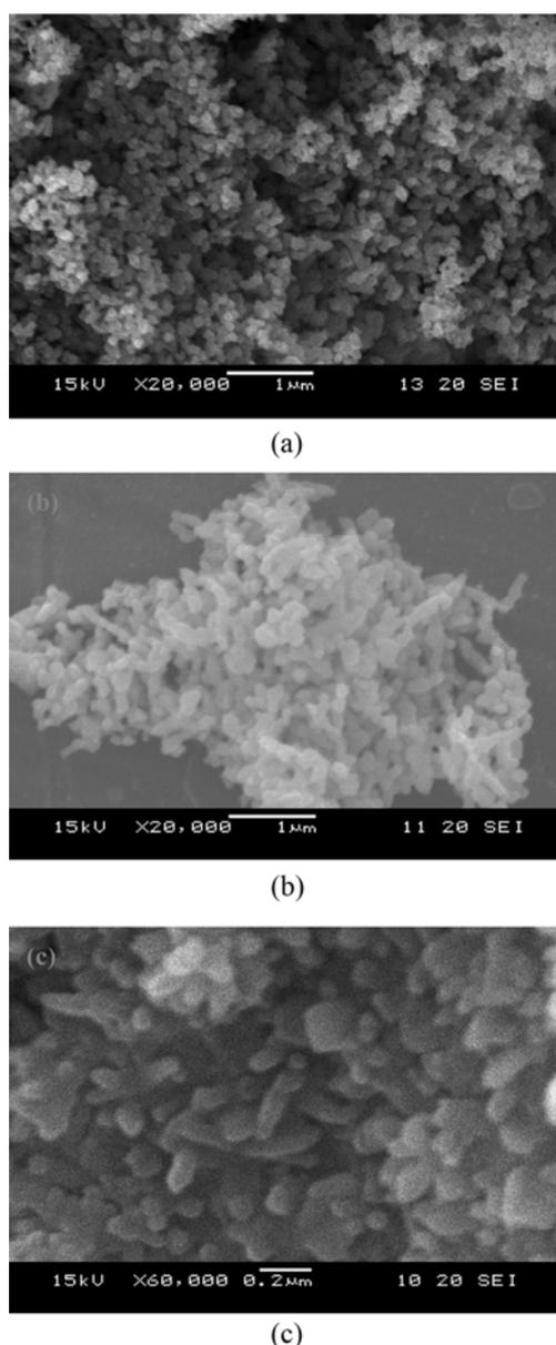
**Fig. 4.** SEM images of ZnO nanoparticles prepared by different methods: (a) direct precipitation using  $\text{Zn}(\text{NO}_3)_2/(\text{NH}_4)_2\text{CO}_3$  as raw materials, (b) sol-gel using  $\text{Zn}(\text{COOCH}_3)_2 \cdot 2\text{H}_2\text{O}/(\text{CH}_3\text{COOH})_2$  as raw materials, (c) a hydrothermal method using  $\text{Zn}(\text{NO}_3)_2/\text{NaOH}$  as raw materials.
