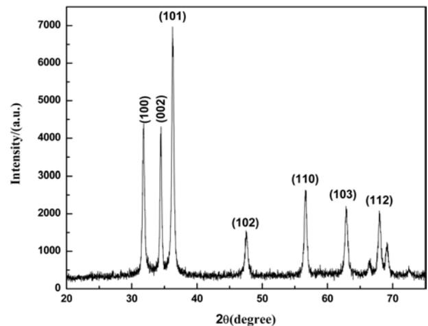
**Fig. 3.** XRD pattern of ZnO nanoparticles prepared by a hydrothermal method.
