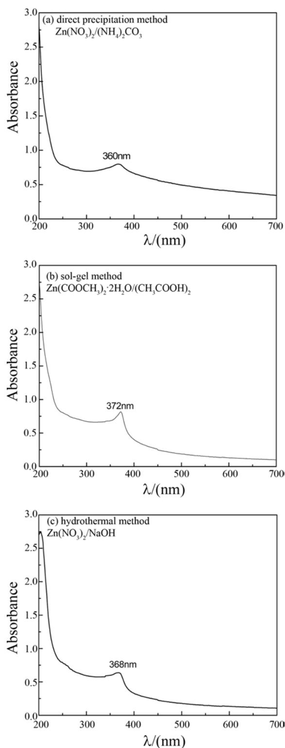
**Fig. 5.** The UV-Vis diffuse reflectance spectra of the ZnO nanoparticles prepared by different methods: (a) a direct precipitation method, (b) a sol-gel method, (c) a hydrothermal method.
