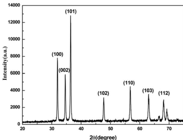
**Fig. 2.** XRD patterns of ZnO nanoparticles prepared by a sol-gel method.
