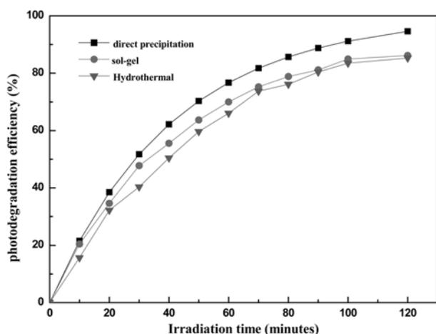
**Fig. 6.** Effect of ZnO nanoparticles prepared by different methods on the photodegradation of methyl orange.
