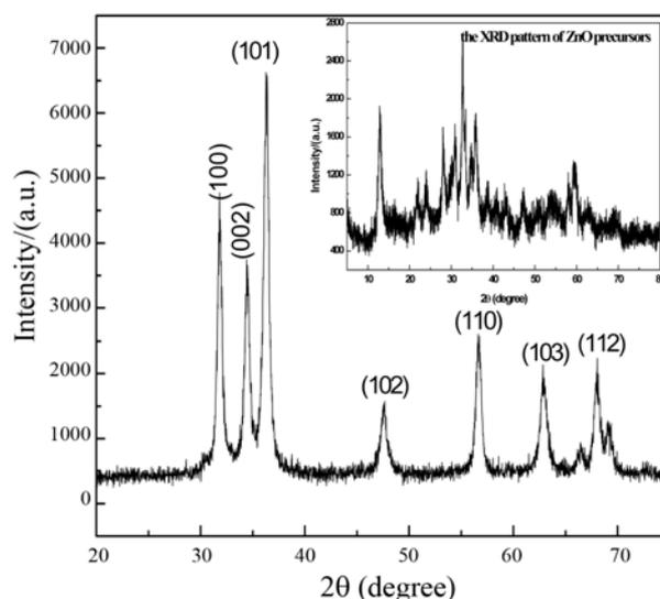
Fig. 1. XRD patterns of ZnO nanoparticles prepared by a precipitation method and the XRD pattern of ZnO precursors in the inset.
